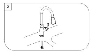
Place optional Escutcheon and Base Plate on bottom of new faucet before position faucet through mounting hole.
