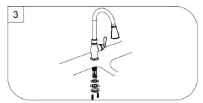
Remove the 2 screws from locking nut .From under the sink,install the rubber washer,steel washer,and locking nut onto the shank Tighten the locking nut with a basin wrench or socket tool and install the 2 screws to secure the faucet in place.
