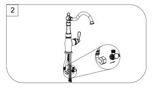
Remove T-Tube from the Inlet hose with adjustable wrench.
