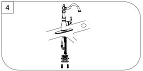
Open the package of mounting kit .Remove the 2 screws from locking nut .From under the sink,install the rubber washer,steel washer,and locking nut onto the shank Tighten the locking nut with a basin wrench or socket tool and install the 2 screws to secure the faucet in place.
