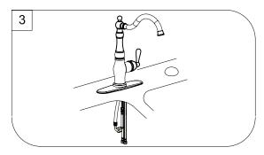
Place optional Escutcheon and Base Plate on bottom of new faucet before positioning faucet through mounting hole.
