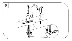
Mount side spray support in far right hole in sink. Insert spray hose down through the support . Attach spray hose to T-tube right threads with wrench.
