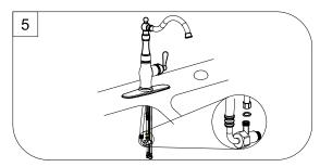
Connect the inlet hose and T-tube left threads(1/2 IPS) with wrench, Then conncet the other end of connector hose to the top threads of T-tube with wrench, ensure the washer is in place. Do not overtighten.
