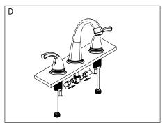
D. Position the bodies as in illustration to install 9.8" flexible water supply hoses on hot and cold inlets. Screw the hose nuts onto the T-tube and tighten firmly. Carefully bend the hoses to fit available space
