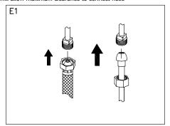
E1. Stainless Steel Brainded Faucet Supply Tubes: This is the simplest of all installations. If you are using stainless steel braided faucet supply tubes, this faucet requires one end of the supply tube to have a 1/2" female IPS connection. The other end of this supply tube must match the thread on the water supply fittings or shut off valve under the sink. Once you have identified the required tube, carefully follow the manufacturer's installations for each tube
