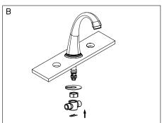
B.Place the spout into center hole of the sink.From under sink Secure firmly to sink with metal washer and nut.Push the T-tube onto the end of the spout tube until it seats.(Caution:There are two O-RING that must seat firmly into the indentations provided on the spout casting.) Insert ring through the groove of the spout tube end.Make sure "T" inlets are aligned at an angle which will allow maximum dearance to connect hose
