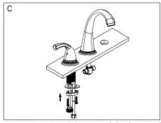
C. Insert the body with the hot supply label is on the(hot) side. Hold the body in the proper position. Assemble metal washer and mounting nut onto body underside of sink, tighten it with the locking screw.
